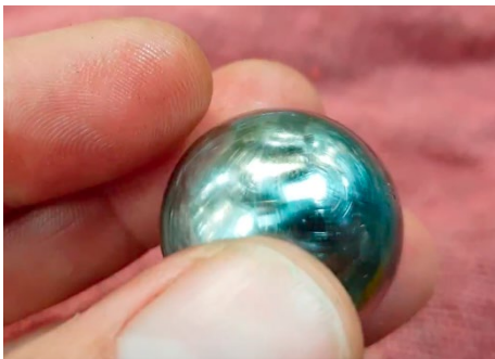
Many circular scars all over the surface of the ball indicated skidding.
