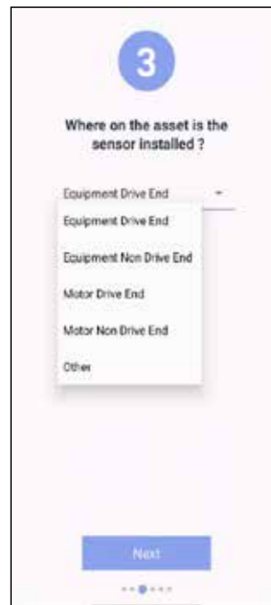
Figure 32: Identifying the sensor location on the equipment
