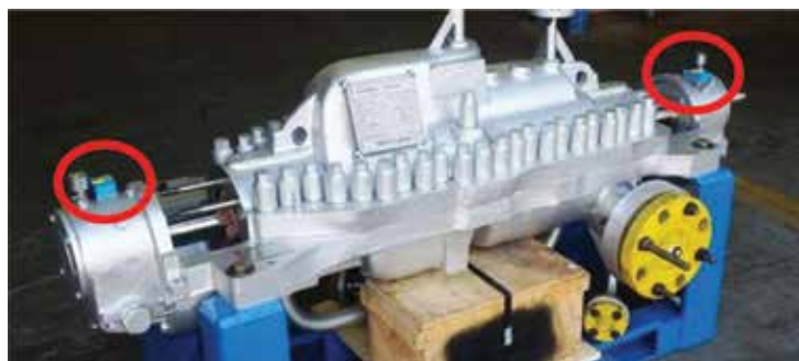
Figure 17: Between Bearings Pump (BB3), mounted on each bearing housing
