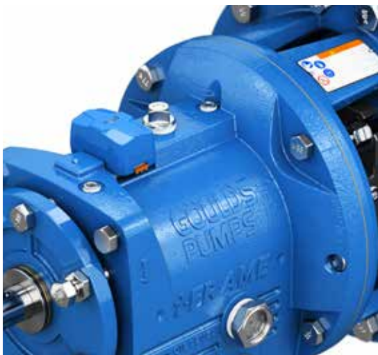
Figure 12: ITT Goulds Pumps 3196 i-FRAME contains mill slot for mounting the monitor
