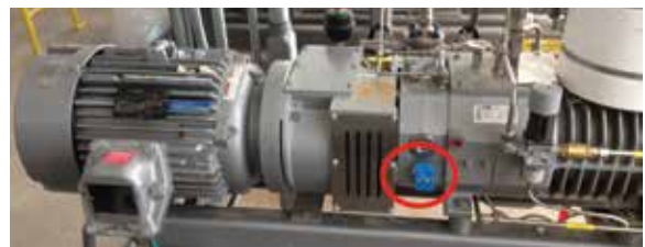
Figure 13: PD pump, side mounted to frame
