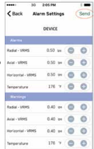
Figure 89: use the + and - buttons to adjust values. Tap "Send" to program the new device settings.
