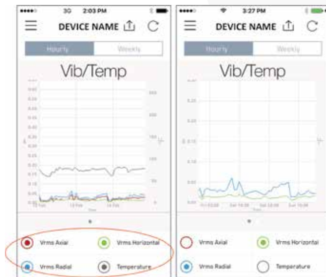
Figure 74: Default Trend view on left, trend view with several measurement de-selected shown on the right.
