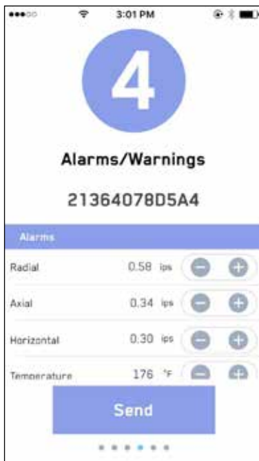
Figure 40: Setting manual alarm levels
