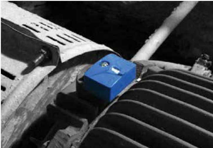
Figure 15: Horizontal motor, mounted over drive end bearing housing
