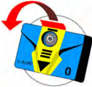
Figure 10: i-ALERT ® 2 Equipment Health Monitor activation
