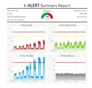
The i-ALERT revealed radial vibration increasing over time.
