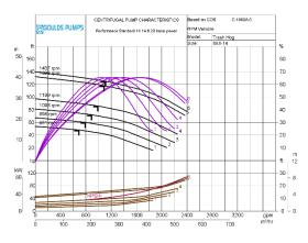
This plot of the system curve against the variable speed curve of the pump revealed a restrictiveness at 1600 gpm.
