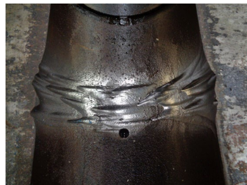
Severe wash out found at mechanical seal areas.
