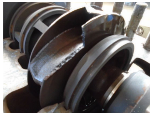
Large piece of impeller found missing and went through pump
